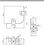
Used for positioning the upright in a corner.
