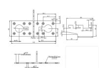
Used when two cabinets are installed side by side. Provides a strong connection.
